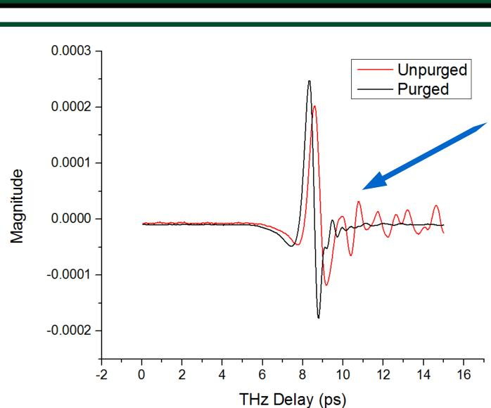
oscillations and low amplitude are due to water absorption Water absorbs THz at particular frequencies
